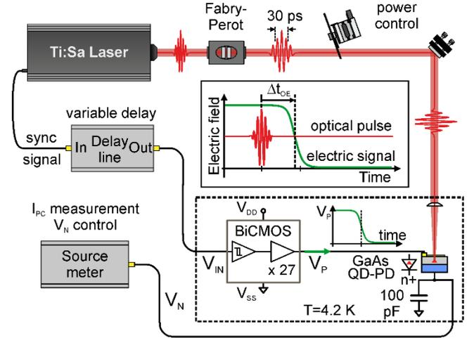
**Fig. 2: Experimental set up for electric chirp experiments. The low capacitance QD photodiode and the ultrafast BiCMOS chip are cooled down to liquid helium temperature. The delay line controls the timing between the optical and electric pulses.**
