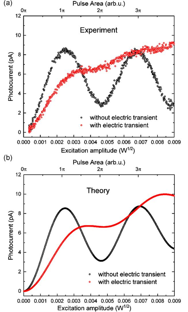
**Fig. 4: Photocurrent corresponding to the occupancy of the two level system as a function of pulse area (a) Experimental data for conditions with (red) and without (black) applied electric transient. (b) Theoretical results corresponding to the experimental conditions.**
