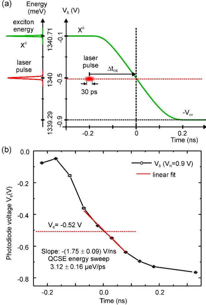
**Fig. 3: Scheme of electric chirp experiment using transform limited optical pulses and ultrafast electrical transients. (a) Tuning of the exciton energy by the applied electric transient (green) with respect to the constant laser energy (red) (b) Electric transient obtained by photocurrent-based sampling of the time-dependent exciton energy as a function of the optoelectronic delay of 30 ps.**
