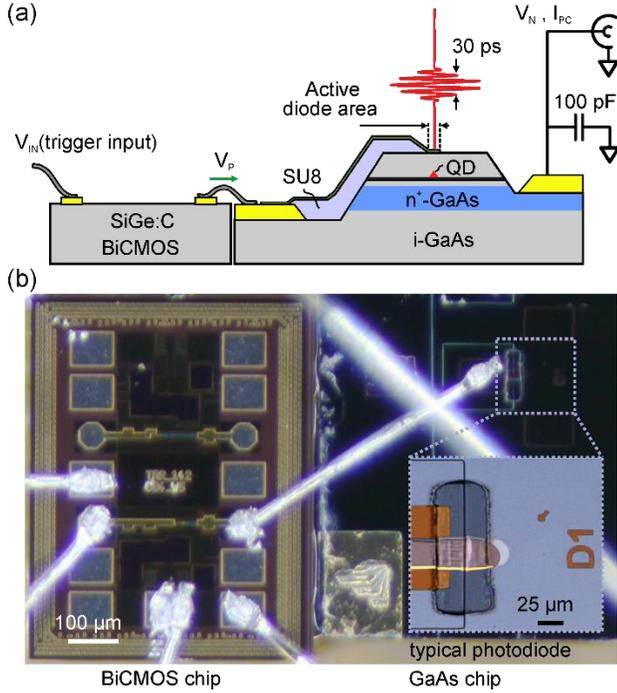
**Fig. 1: System integration of an ultrafast electric BiCMOS chip and a low capacitance QD photodiode. (a) Schematic layout of the connected electrical chip and the GaAs photodiode sample in cross-sectional view. (b) Photograph of the used BiCMOS chip connected to a GaAs QD photodiode.**
