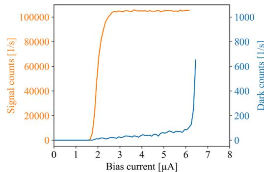
Figure 4. Measured signal counts of an integrated SNSPD showing a saturation plateau, as well as noise counts (dark counts) for different detector bias currents.
