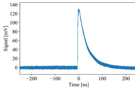
Figure 3. Measured detector response of an integrated SNSPD.
