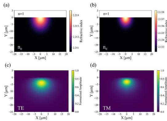
**Figure 1.** Modelled refractive index distribution of titanium in-diffused waveguides at 1550 nm wavelength for light in TE polarization seeing the ordinary refractive index in (a) and TM polarization seeing the extraordinary refractive index in (b). Corresponding simulated waveguide modes are shown in (c) and (d).
