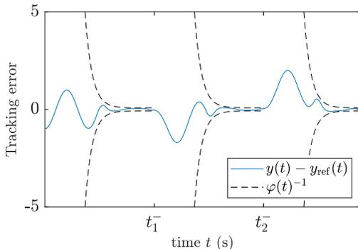
Fig. 4: Error between the output  $y$  and the reference signal  $y_{\text{ref}}$ ; and funnel boundary  $1/\varphi$ .
