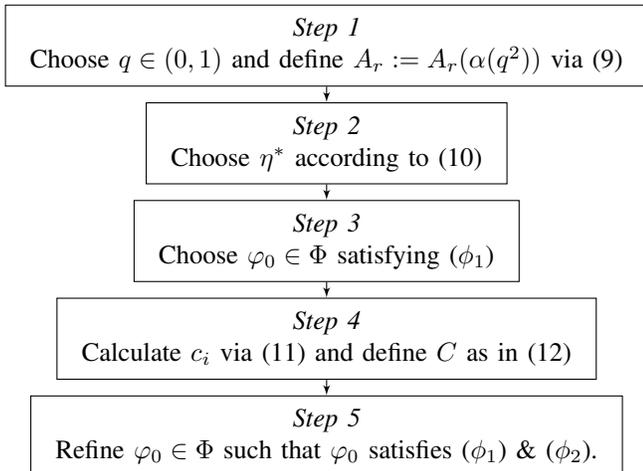
Fig. 1: Flowchart for the choice of the controller design parameters.
