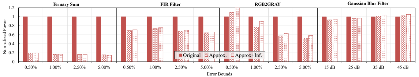
Fig. 4: Power results for original, approximate and approximate+infected of four most commonly used benchmarks
