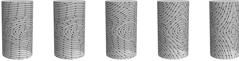
Figure VIII.6: Phase portrait of the Eringen's nonlocal elastica for \beta = 1 , l = 0 , l = 0.2 , l = 0.5 , l = 0.7 and l = 0.9
