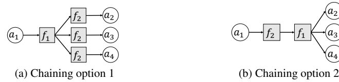
Figure 3. Two different options for the structure of an example service, consisting of two VNF types f_1 and f_2 that can be traversed in an arbitrary order between the endpoints
